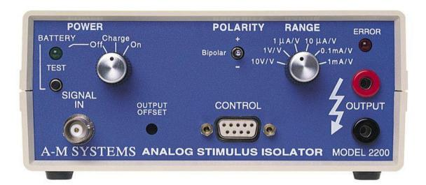
The Model 2200 Analog Stimulus Isolator is designed for a wide variety of applications. It provides opto-electrical isolation for stimuli generated by a wide range of signal sources. The signal is DC-coupled, and can take on any waveshape within its wide bandwidth.
